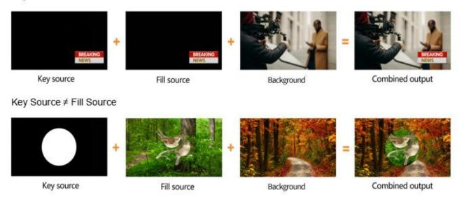
Luma key provides a way to composite a Text clip over a background clip based on the luminance levels in the video. Turn on the Luma Key, a color from the key source will be removed, revealing another background image behind it.
