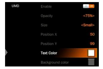
The UMD content for each SDI and HDMI input can be set from the on-screen menu. The user can use a virtual keyboard and rotary button to rename the UMD content for each window. The UMD content can be up to 10 characters long. Below image as an example, rename the IN1 to CAM1.
